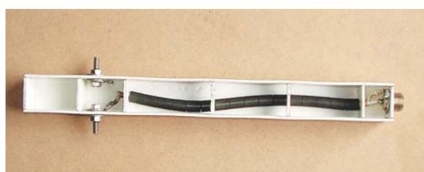
Photo 2: The coaxial cable choke.
